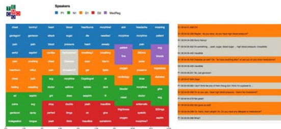
Figure 5. The TeMoCo prototype, with a speaker turn selected on the visualization (grayed out mosaic on the left), and the relevant parts of the transcripts highlighted (orange background text on the right).
