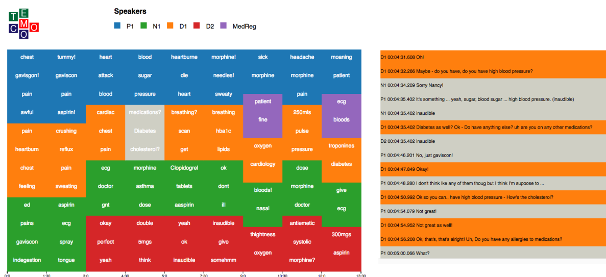
Figure 11: The TeMoCo prototype, with a speaker turn selected on the visualization (grayed out mosaic on the left), and the relevant parts of the transcripts highlighted (orange background text on the right).
