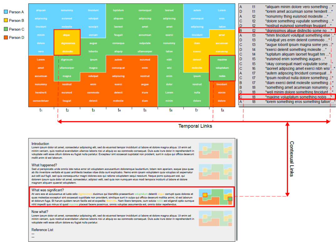
Figure 13: Sketch of the main components of the visualization: temporal mosaic of the audio dialogue (top left) and its transcript (top right), and the related text document (bottom).
